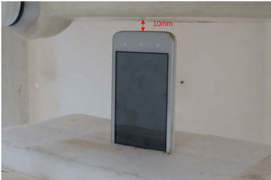
Picture 18: Bottom Edge, the distance from handset to the bottom of the Phantom is 10mm
