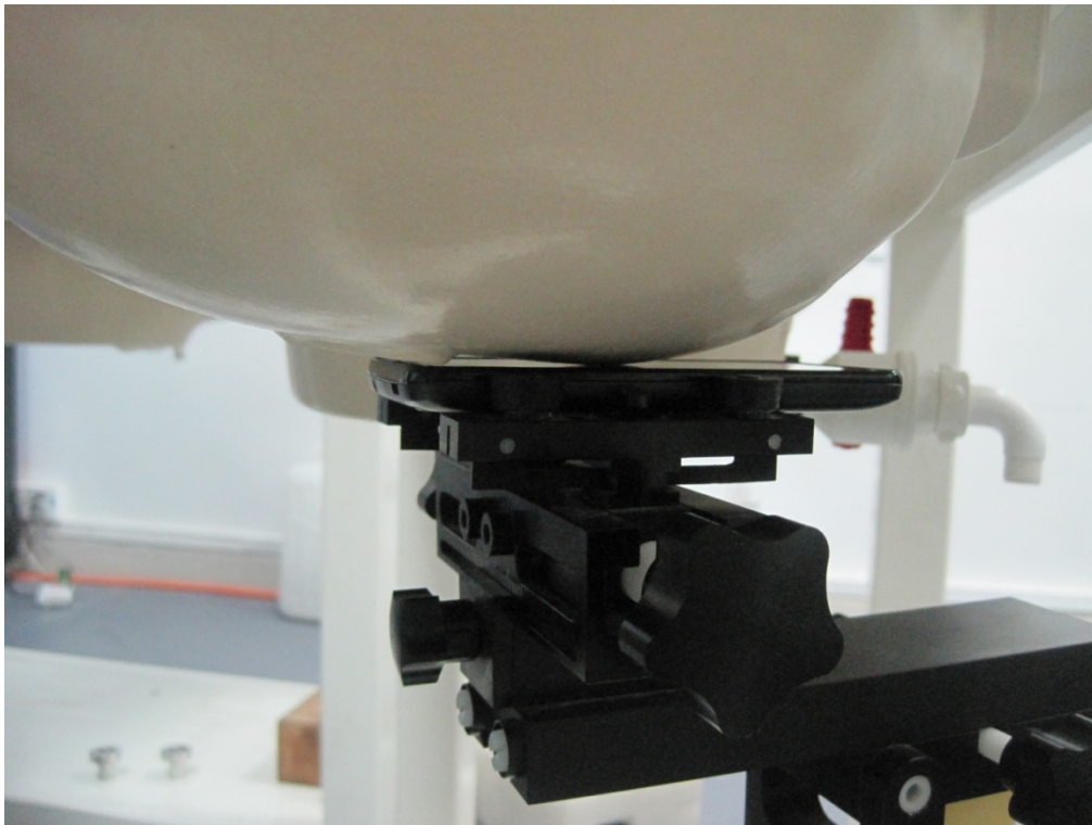
Picture 1-5: Right Hand Touch Cheek Position
