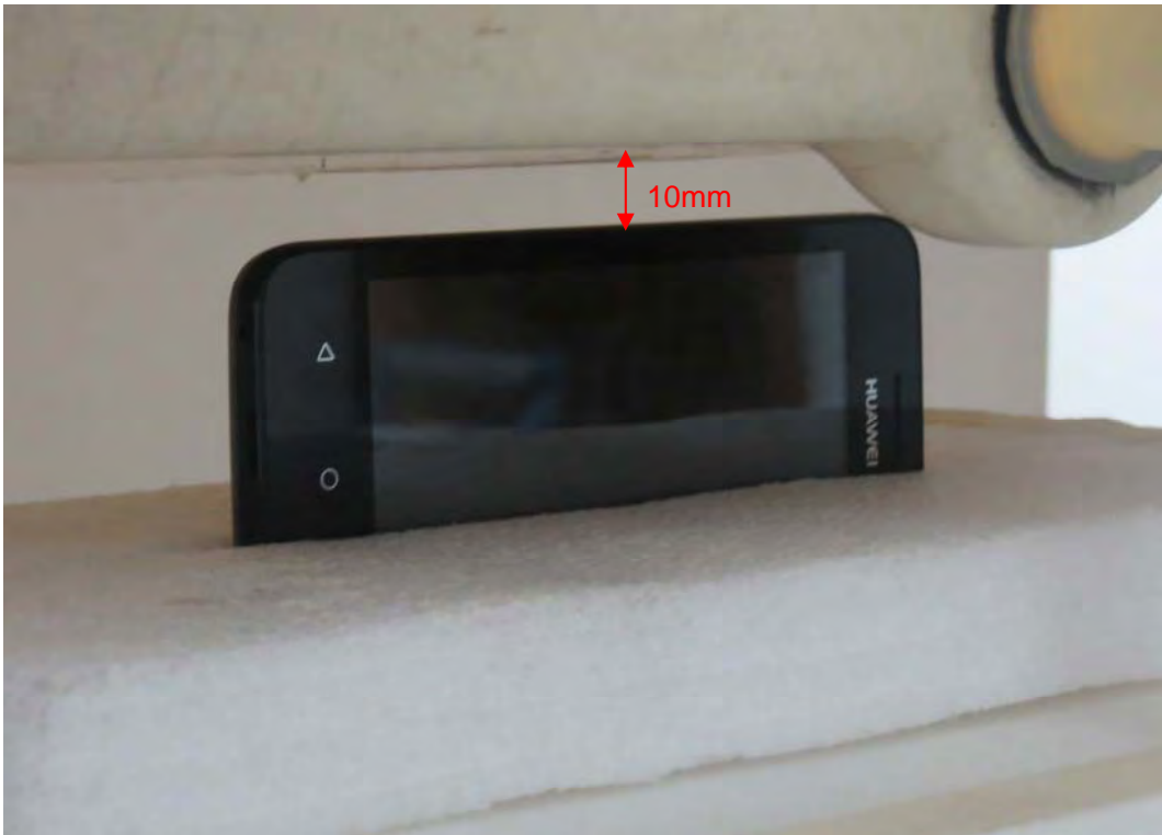
Picture 15: Left Edge, the distance from handset to the bottom of the Phantom is 10mm
