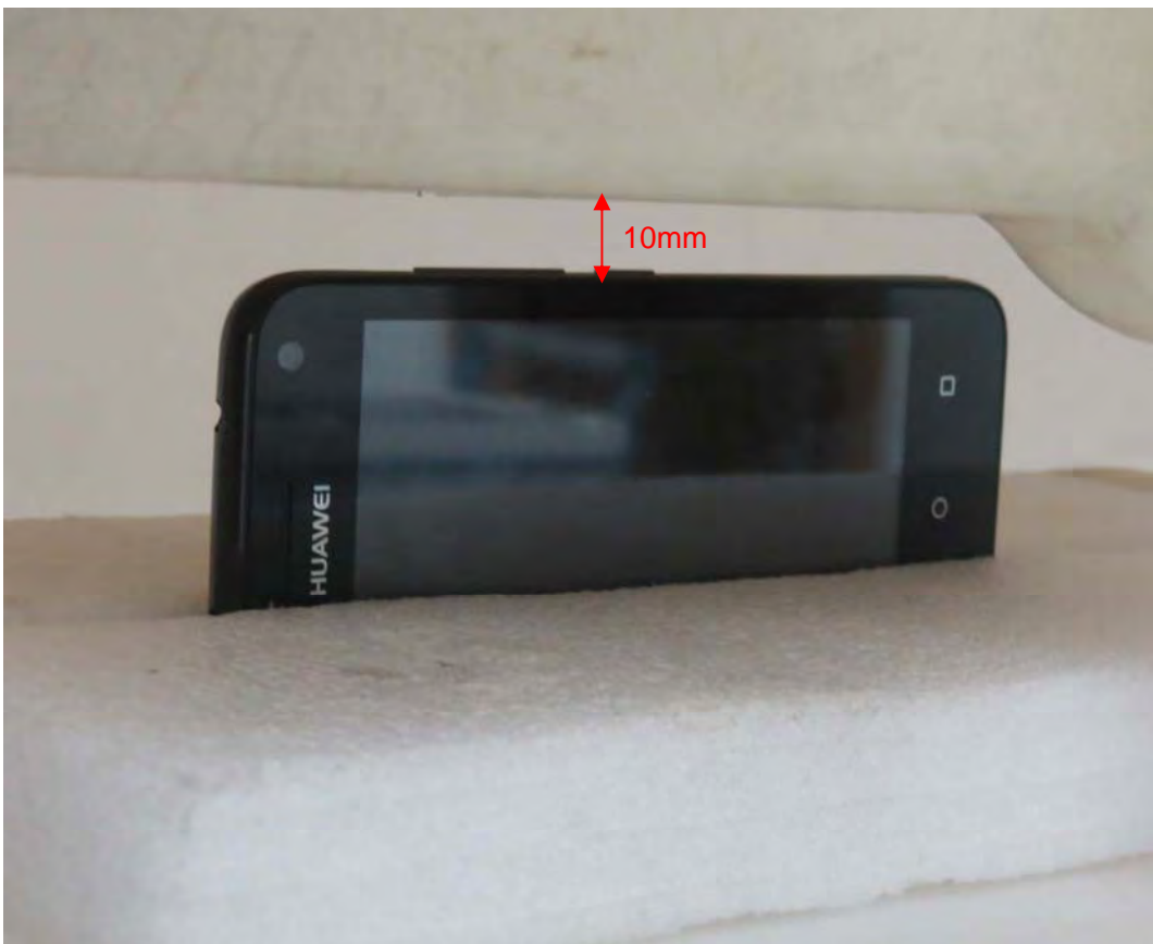
Picture 16: Right Edge, the distance from handset to the bottom of the Phantom is 10mm
