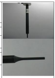
Isotropic E-Field Probe EX3DV4 for Dosimetric Measurements
