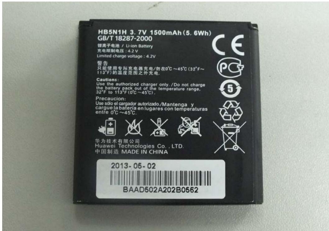
Battery 1 (Main Battery)
