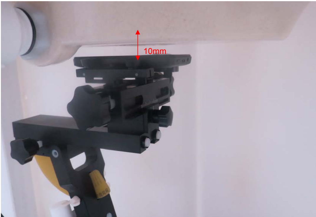
Picture 14: Front Side, the distance from handset to the bottom of the Phantom is 10mm (Original)
