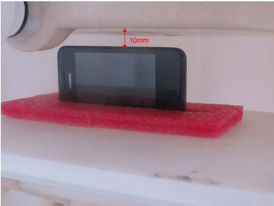
Picture 16: Right Edge, the distance from handset to the bottom of the Phantom is 10mm (Original)
