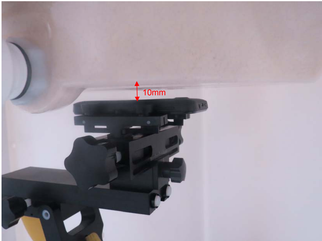
Picture : Back Side, the distance from handset to the bottom of the Phantom is 10mm
