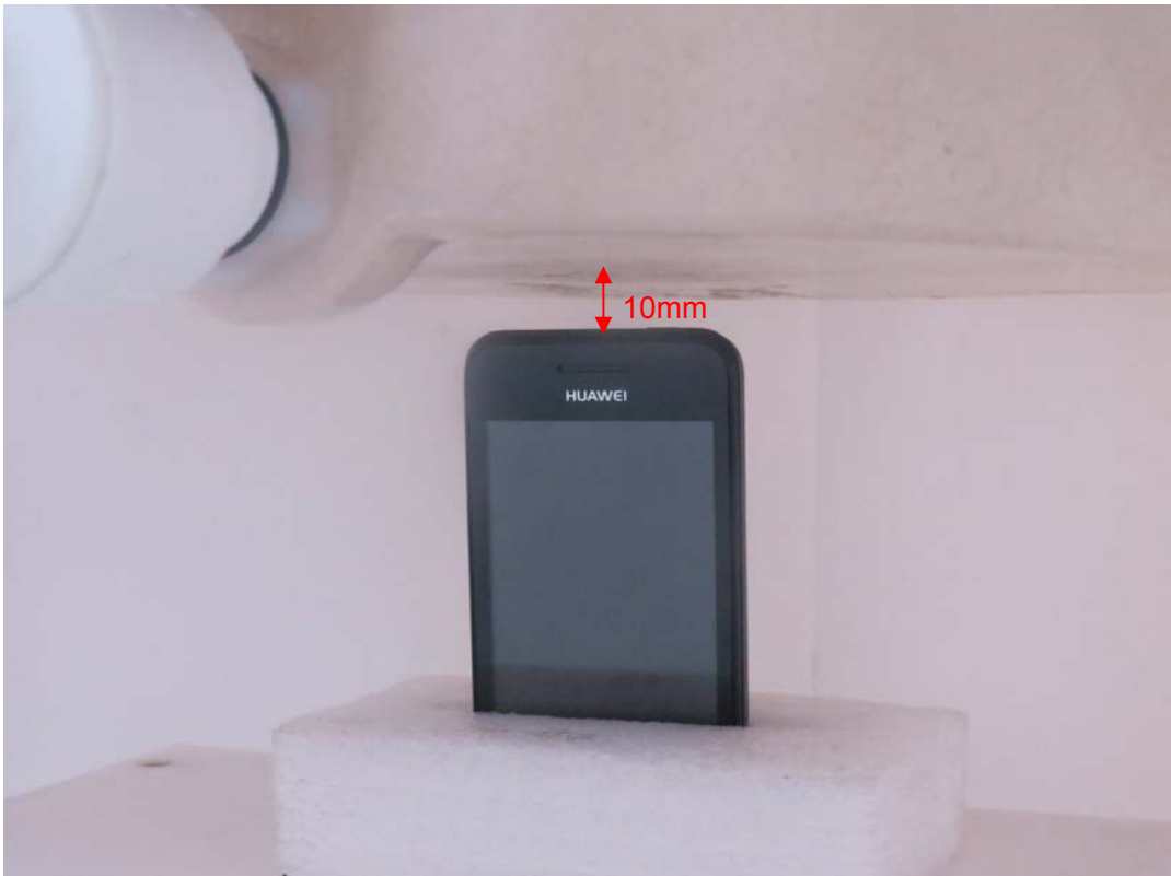
Picture : Top Edge, the distance from handset to the bottom of the Phantom is 10mm
