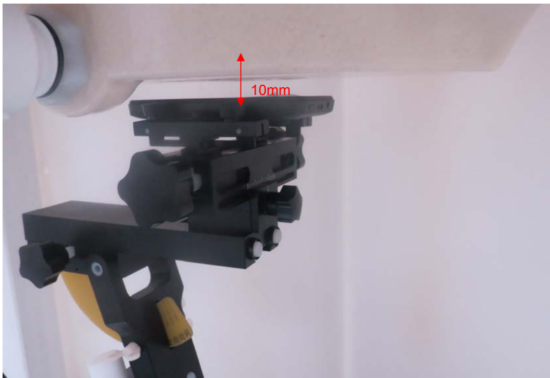
Picture : Front Side, the distance from handset to the bottom of the Phantom is 10mm
