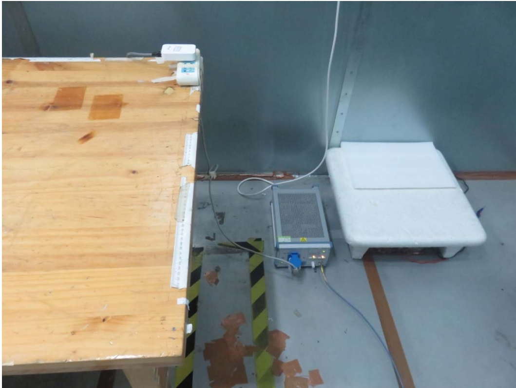
Picture 2 Conducted Emission Test Setup
