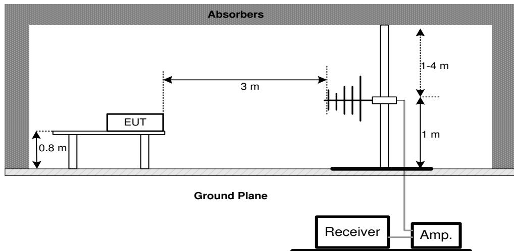
(B) Radiated Emission Test Set-Up Frequency 1 GHz
