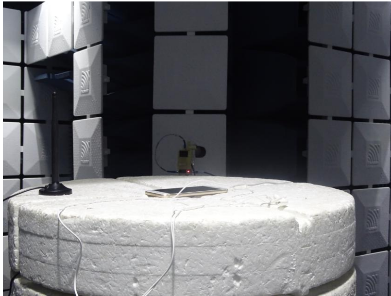
Radiated Spurious Emission (18GHz to26.5GHz)
