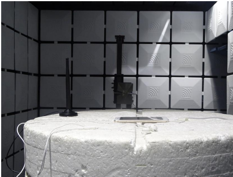
Radiated Spurious Emission (3GHz to18GHz)
