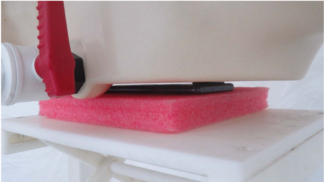
Picture 13: Back Side, the distance from handset to the bottom of the Phantom is 0mm
