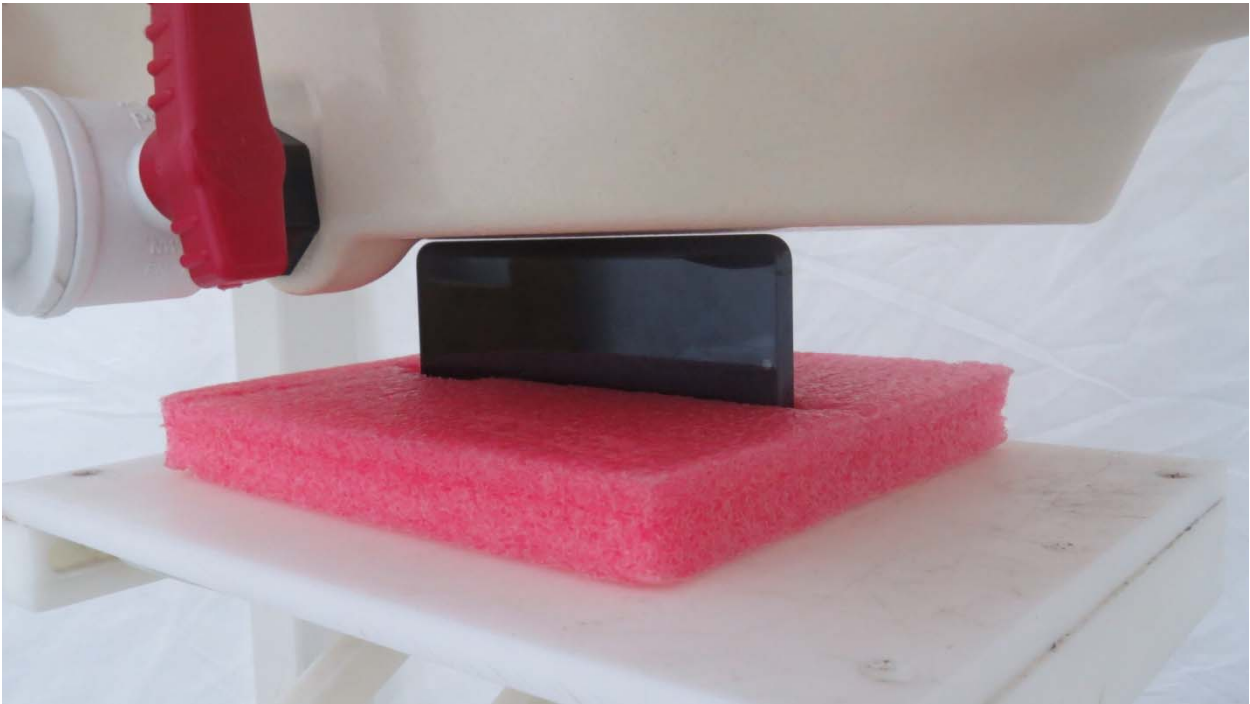
Picture 15: Left Side, the distance from handset to the bottom of the Phantom is 0mm
