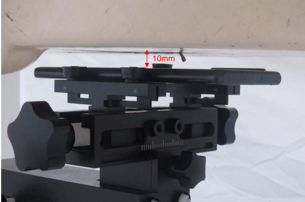
Picture 7: Back Side, the distance from handset to the bottom of the Phantom is 10mm
