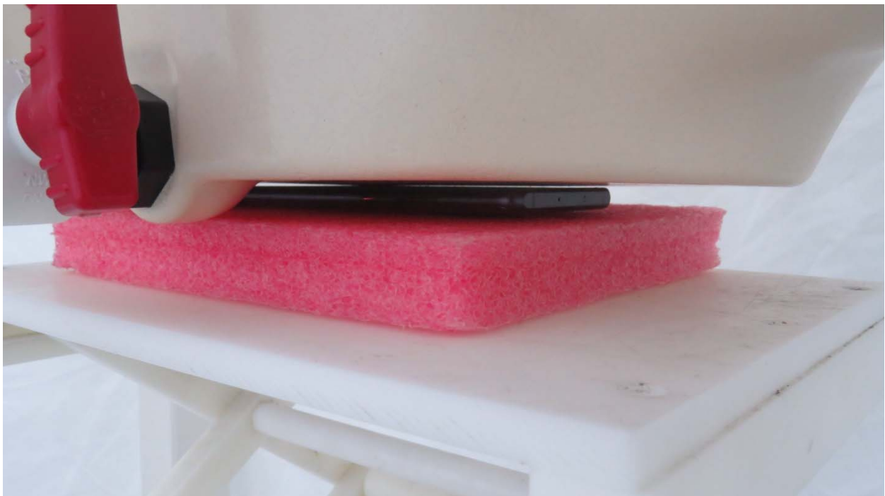
Picture 14: Front Side, the distance from handset to the bottom of the Phantom is 0mm
