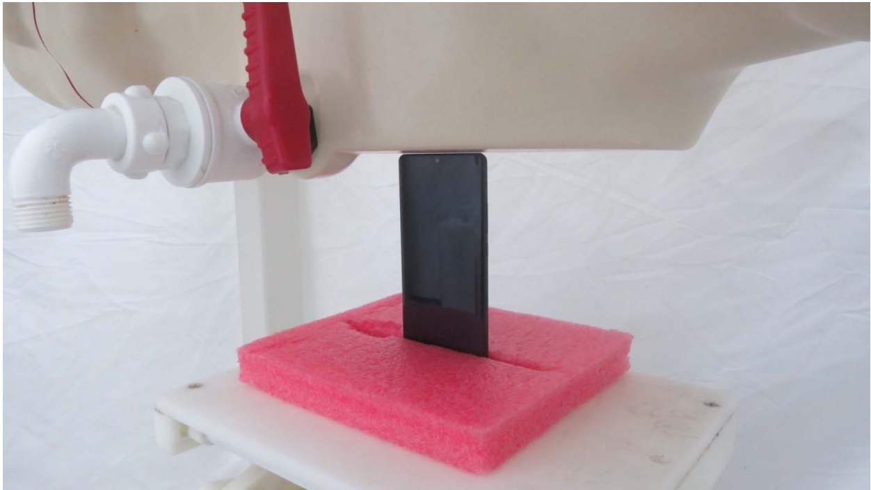
Picture 17: Top Side, the distance from handset to the bottom of the Phantom is 0mm
