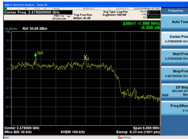
BT UHD 2M \pi/4 -DQPSK CH37, Carrier frequency (MHz): 2478
