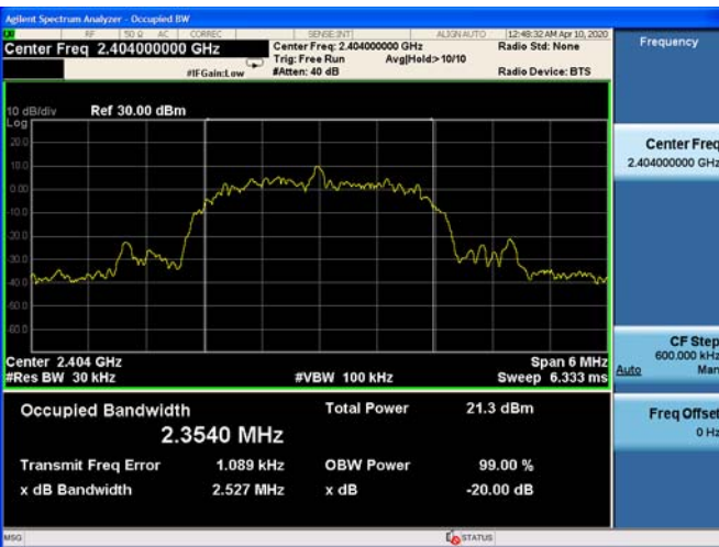
BT UHD 2M \pi/4 -DQPSK, Carrier frequency (MHz): 2440
