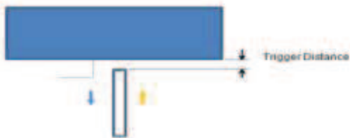
Picture: Proximity sensor triggering distances assessment Bottom Side
