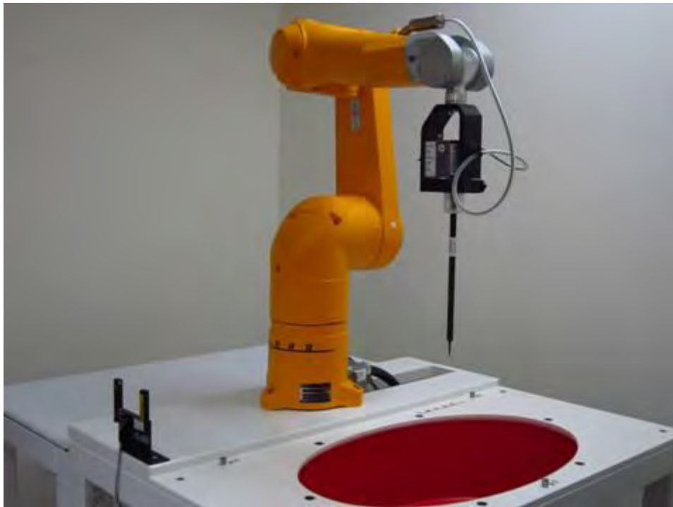
Fig.1 Photograph of the SAR measurement system
