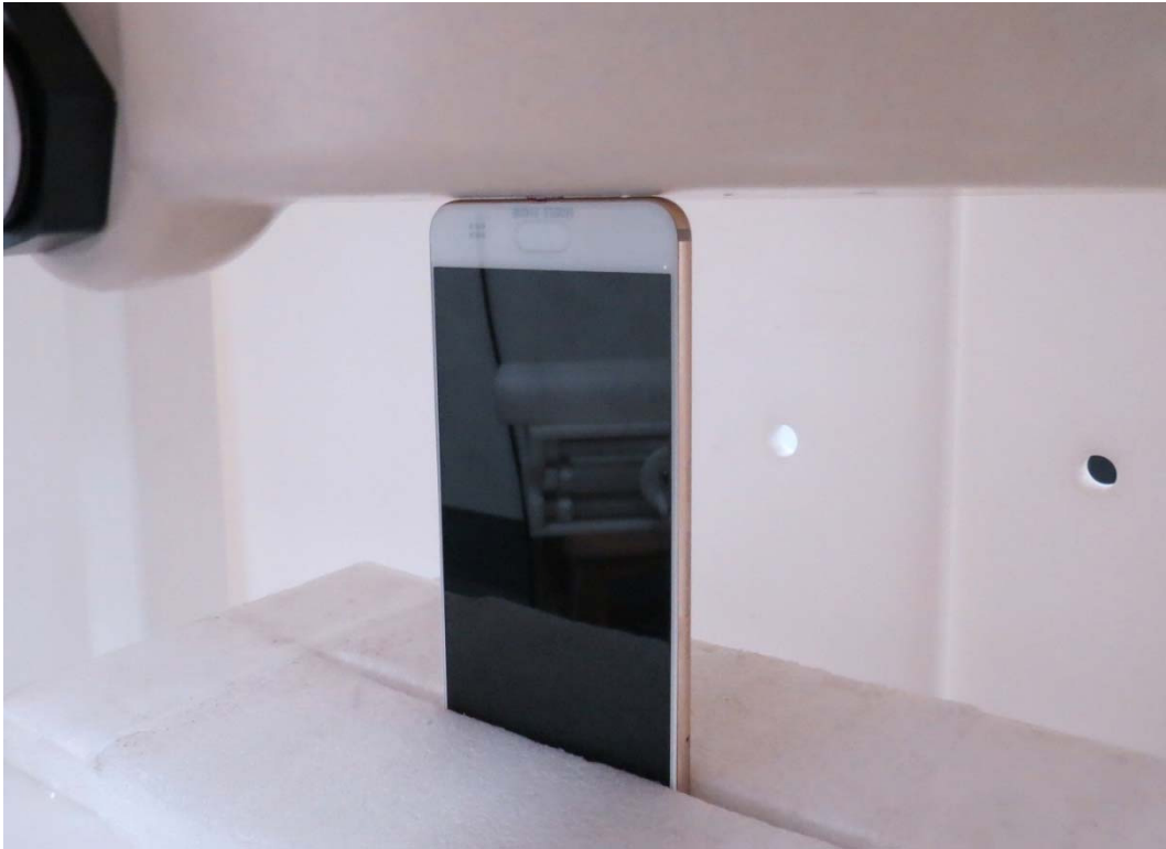
Picture 20: Bottom Edge, the distance from handset to the bottom of the Phantom is 0mm
