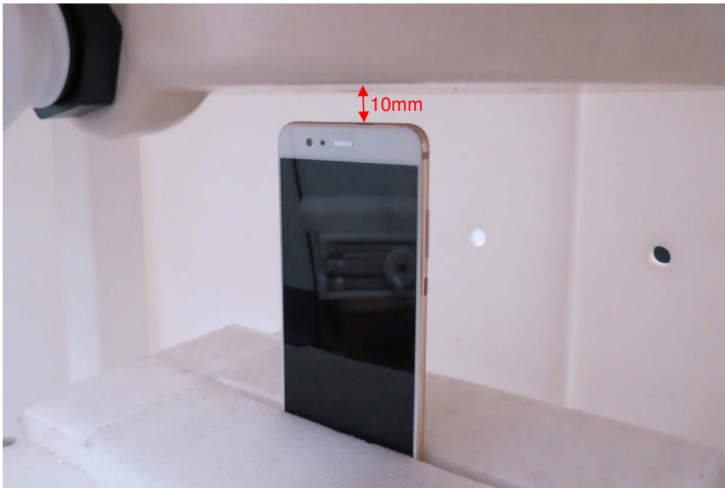
Picture 13: Top Edge, the distance from handset to the bottom of the Phantom is 10mm
