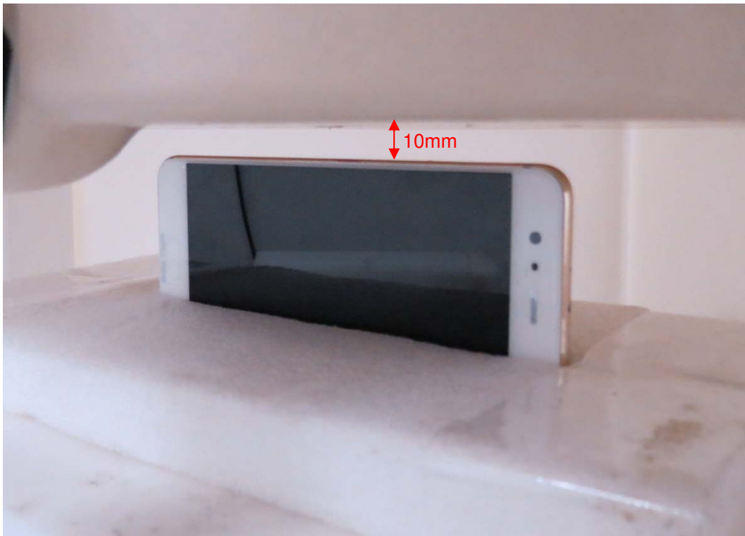
Picture 11: Left Edge, the distance from handset to the bottom of the Phantom is 10mm
