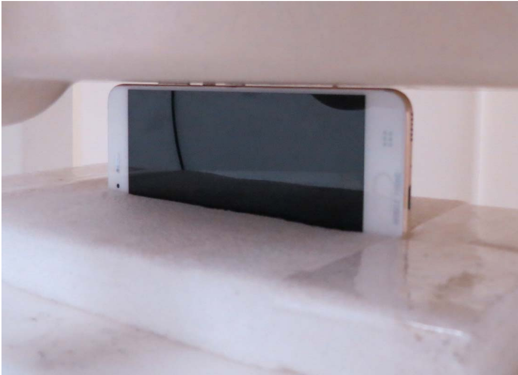
Picture 18: Right Edge, the distance from handset to the bottom of the Phantom is 0mm
