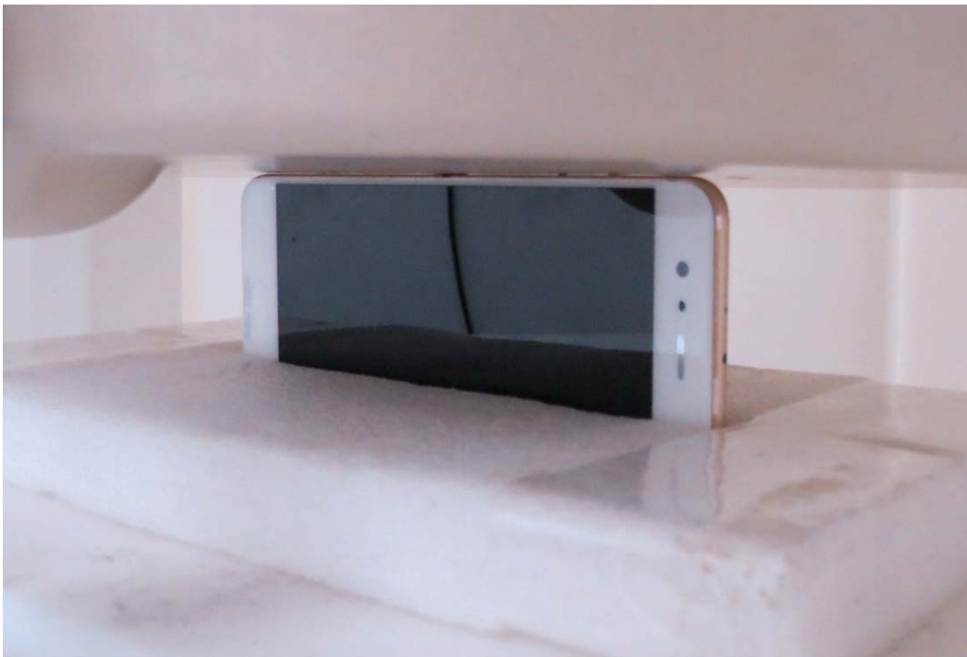
Picture 17: Left Edge, the distance from handset to the bottom of the Phantom is 0mm
