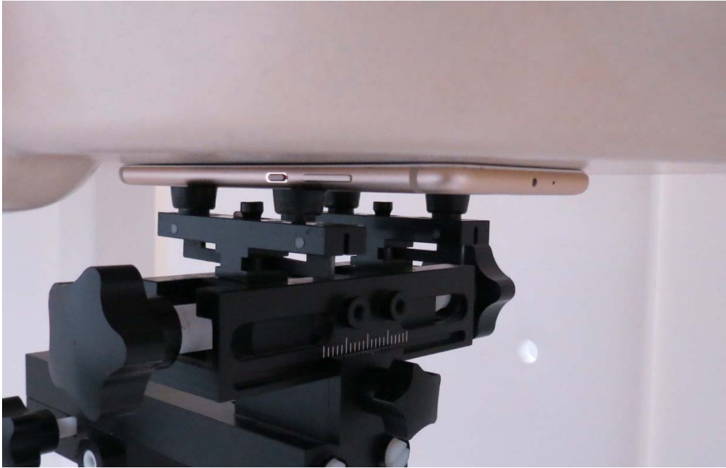
Picture 16: Front Side, the distance from handset to the bottom of the Phantom is 0mm
