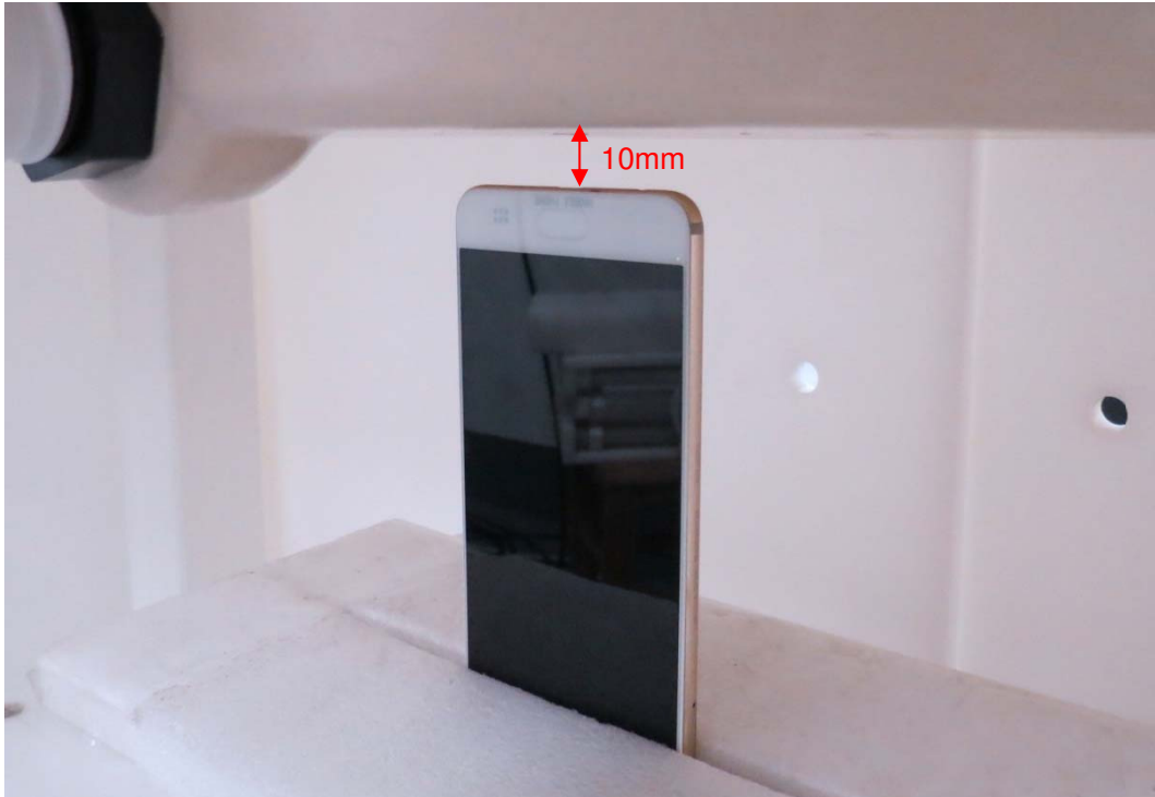
Picture 14: Bottom Edge, the distance from handset to the bottom of the Phantom is 10mm
