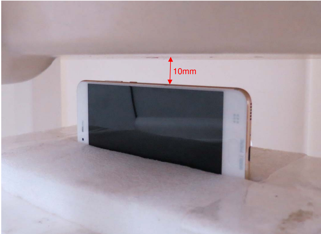
Picture 12: Right Edge, the distance from handset to the bottom of the Phantom is 10mm
