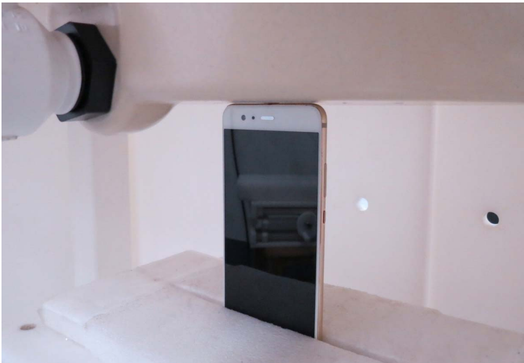
Picture 19: Top Edge, the distance from handset to the bottom of the Phantom is 0mm
