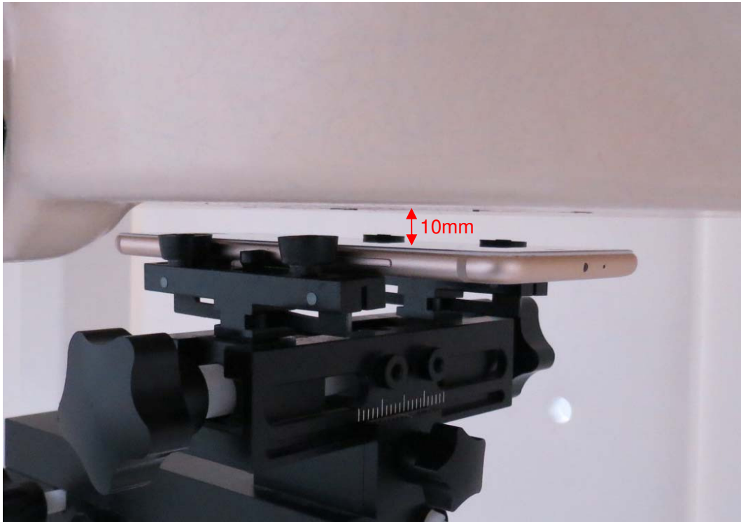
Picture 10: Front Side, the distance from handset to the bottom of the Phantom is 10mm
