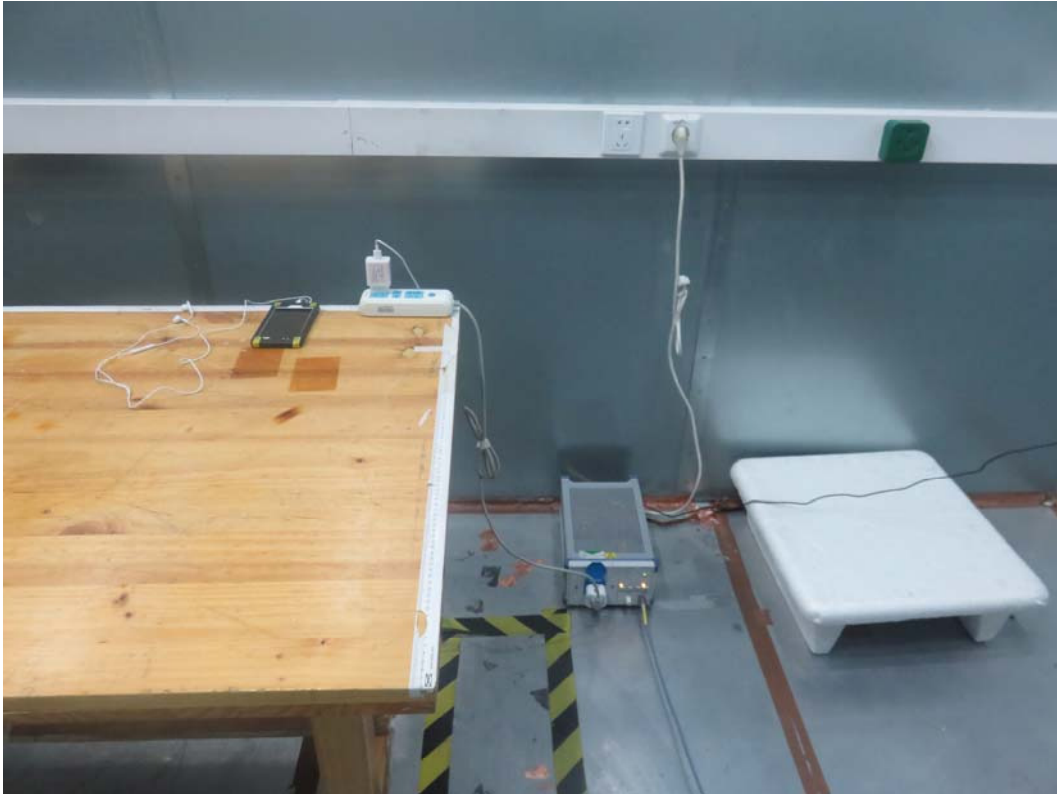
Picture 3 Conducted Emission Test Setup
