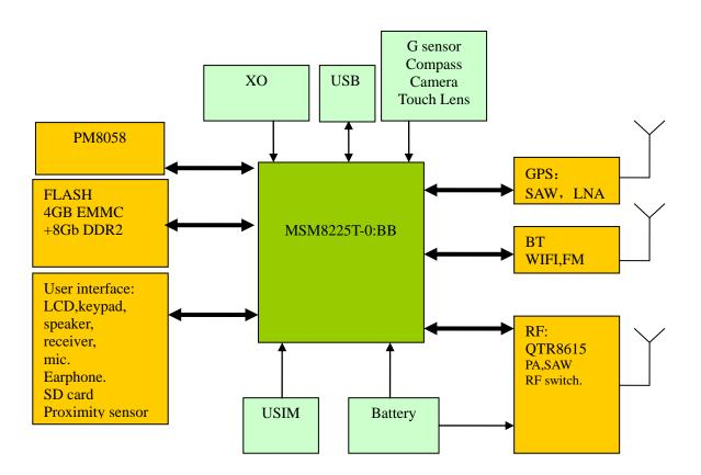
MSM8225T-0:Mobile Station Modem IC PM8058: Power Manager IC QTR8615:Radio Frequency Transceiver BCM4330 :Bluetooth/WIFI/FM IC XO:19.2M Clock
