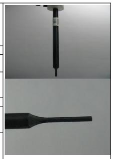
Isotropic E-Field Probe EX3DV4 for Dosimetric Measurements
