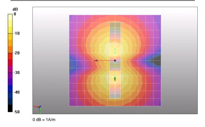
Figure 18 T-Coil WCDMA Band II Y transversal
