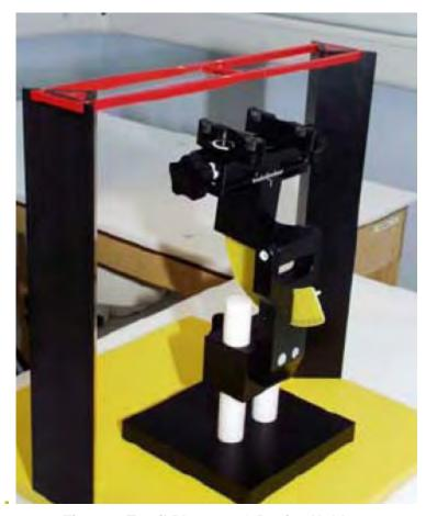
Figure 7 T-coil Phantom & Device Holder
