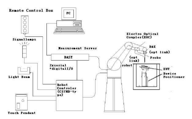
Figure 1 T-Coil Test Measurement Set-up
