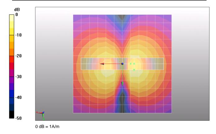
Figure 23 T-Coil WCDMA Band V X longitudinal
