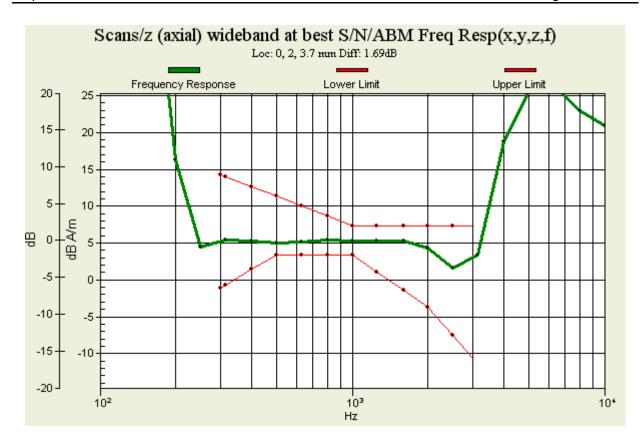
Figure 16 T-Coil GSM 1900 Z Axial
