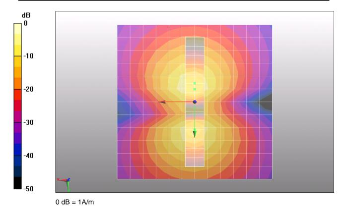
Figure 21 T-Coil WCDMA Band IV Y transversal
