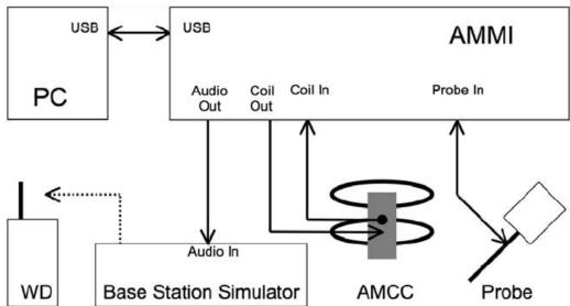
Figure 2 T-Coil Test Measurement Set-up
