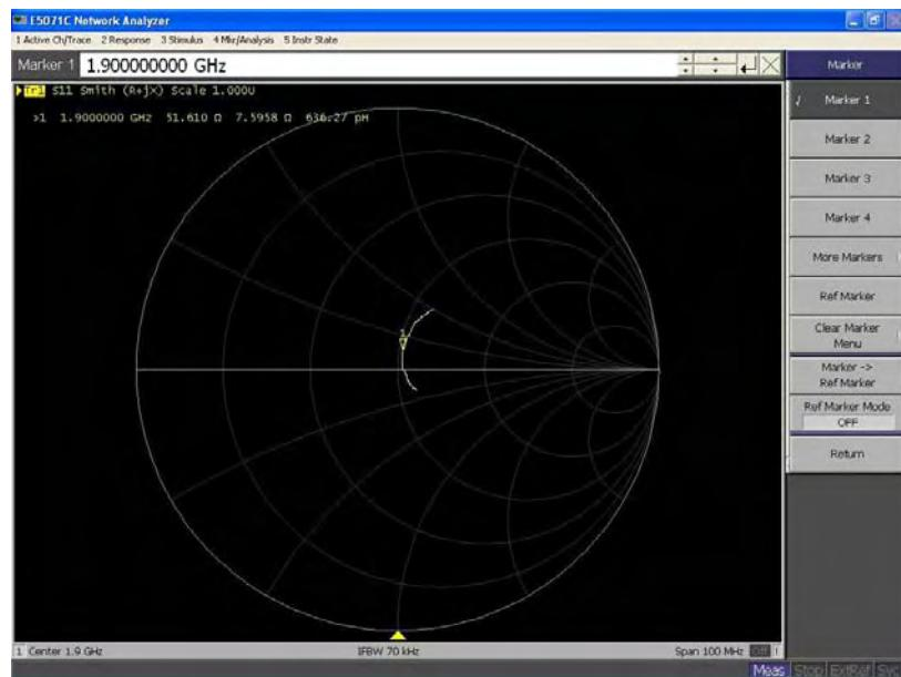
Calibrated return loss: -22.7 dB; Measured impedance: -23.651 dB (within 20%)
