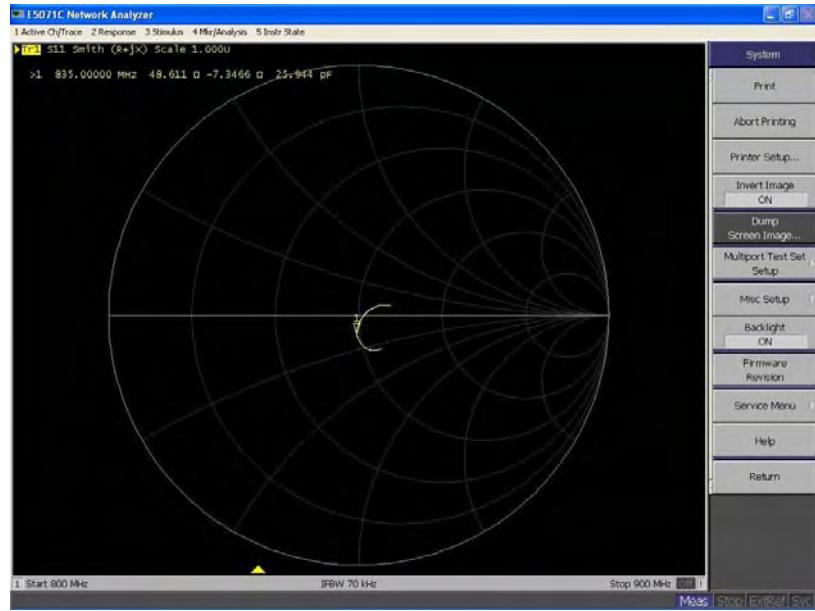
Calibrated return loss: -25.5 dB; Measured impedance: -26.333 dB (within 20%)
