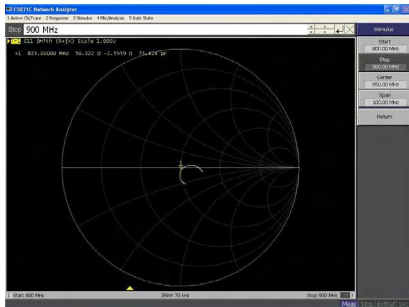
Calibrated return loss: -29.4 dB; Measured impedance: -27.246 dB (within 20%)
