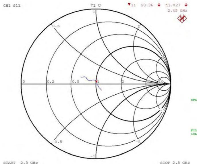
Calibrated return loss: -40.8 dB; Measured impedance: -42.22 dB (within 20%)
