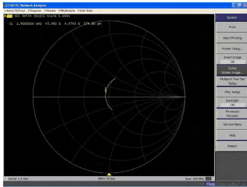
Calibrated return loss: -21.5 dB; Measured impedance: -19.090 dB (within 20%)
