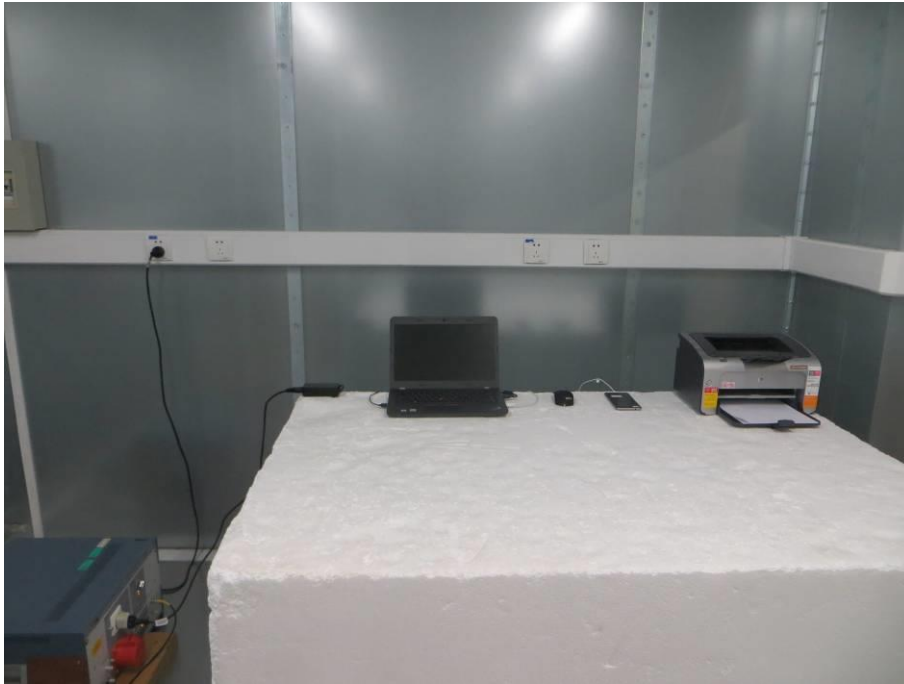
5. Conducted Emission (Part 15B PC mode)
