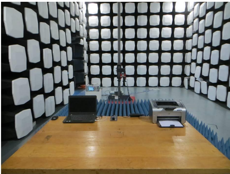
2. Radiated Emissions (Part 15B PC mode)(Above 1GHz)
