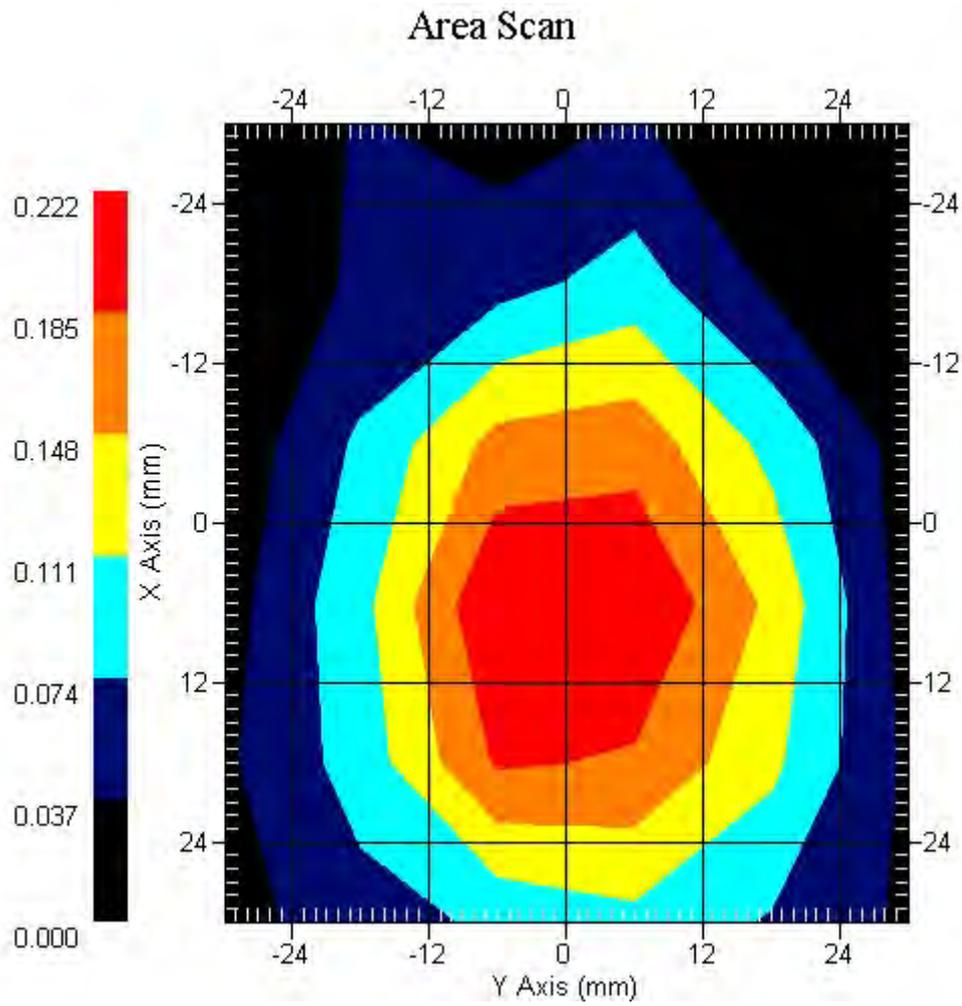
GSM 850 EUT Right Cheek Z-Axis plot
