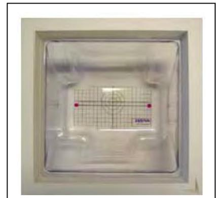
The design allows for fast and accurate measurements, of handsets, by allowing the conservative SAR to be evaluated at on frequency for both left and right head experiments in one measurement.
