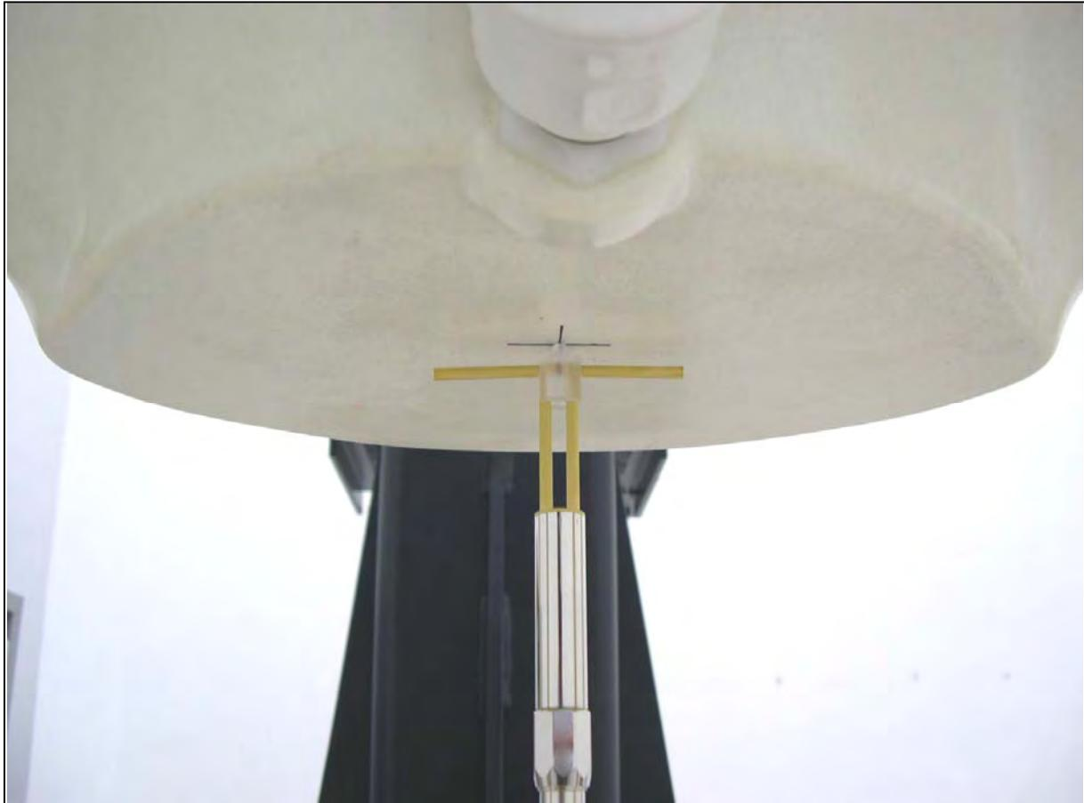
**Fig 8.2 Dipole Setup**
