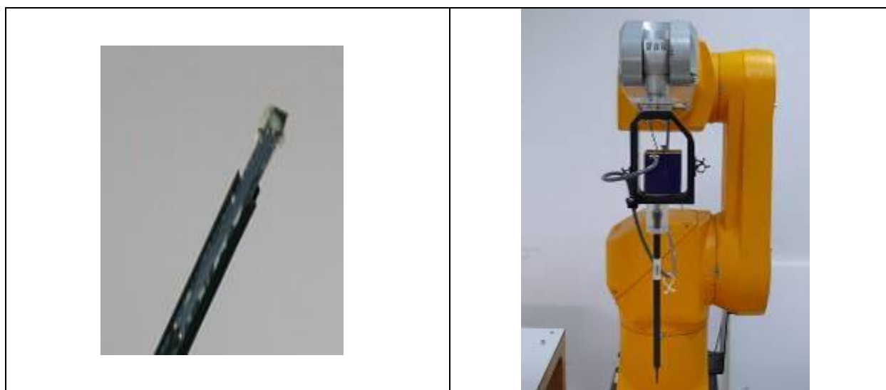
EX3DV4 E-field Probe
