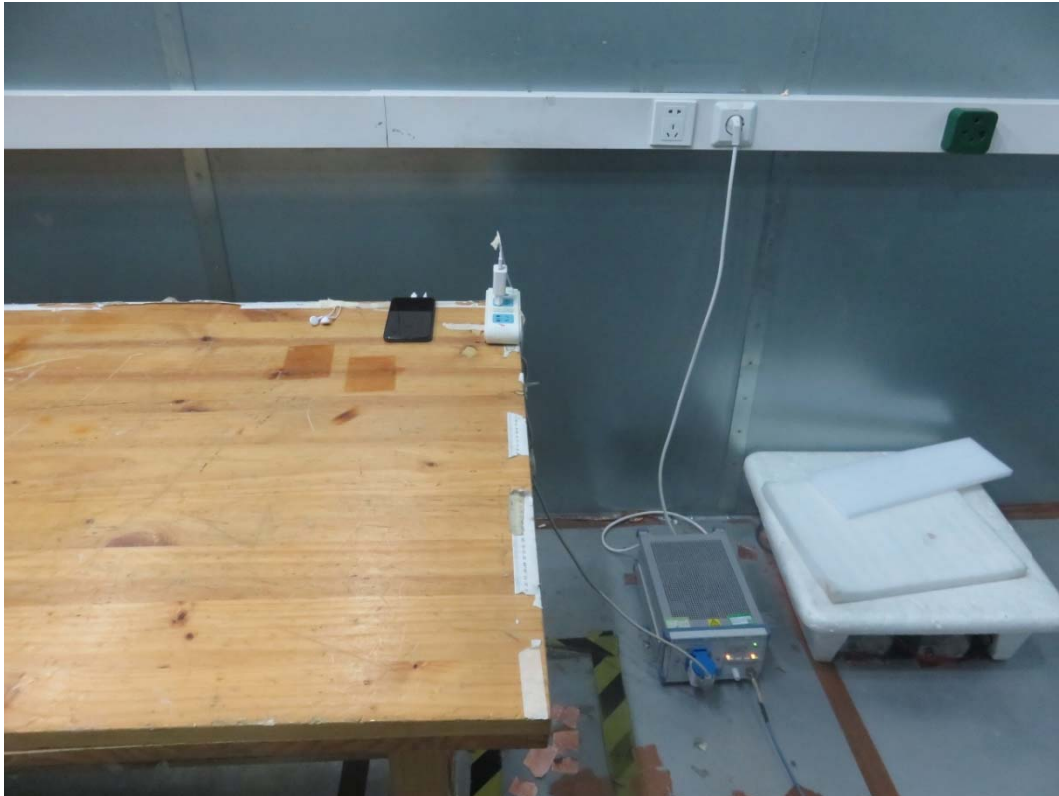
Picture 2 Conducted Emission Test Setup
