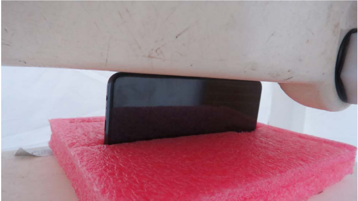
Picture 13: Left Side, the distance from handset to the bottom of the Phantom is 0mm
