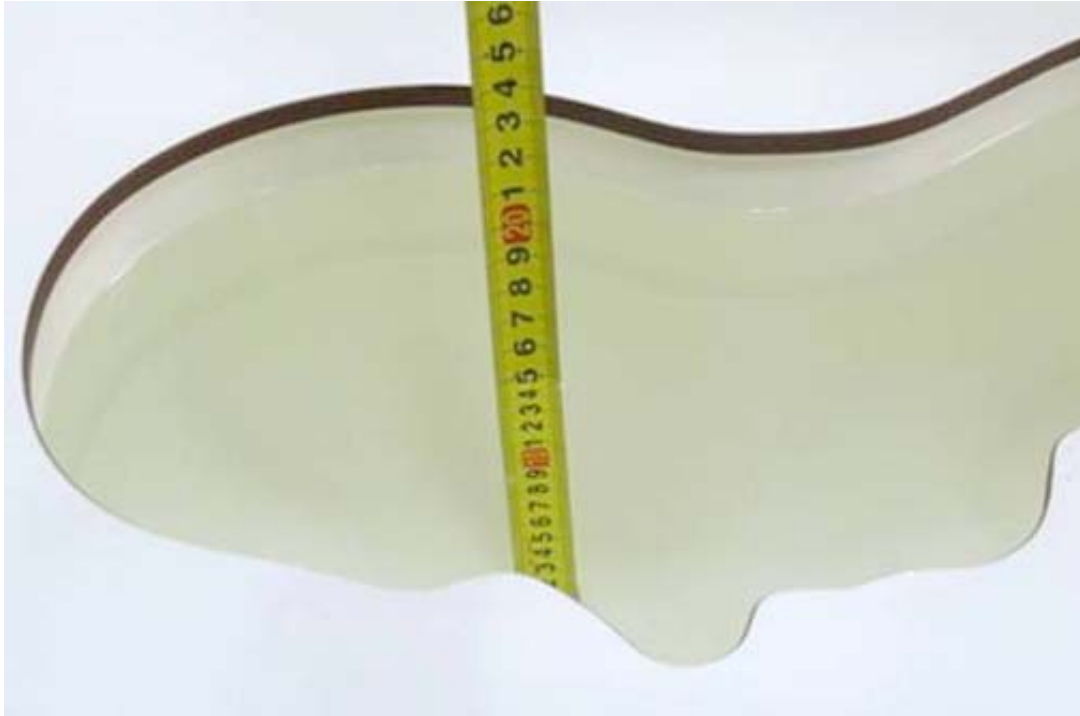
Picture 3: liquid depth in the head Phantom
