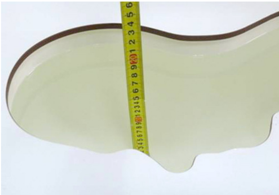
Picture 13: Liquid depth in the head Phantom (5200 MHz, 15.4cm depth)
