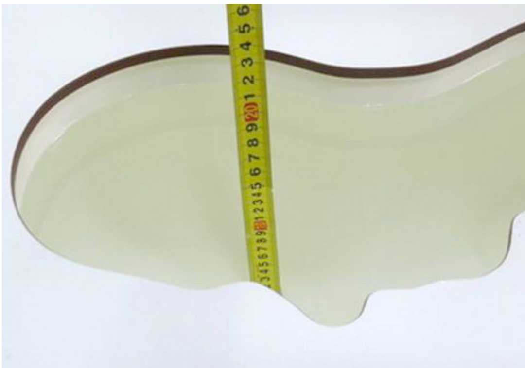
Picture 17: Liquid depth in the head Phantom (5800 MHz, 15.4cm depth)
