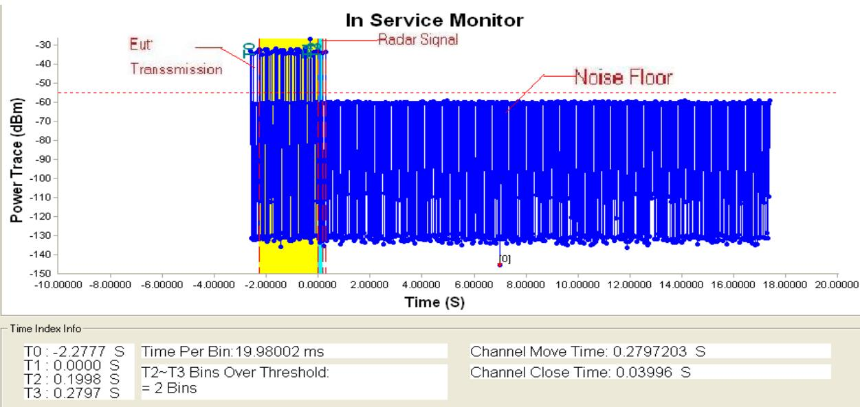
**Note:** T1 denotes the start of Channel Move Time upon the end of the last Radar burst.
