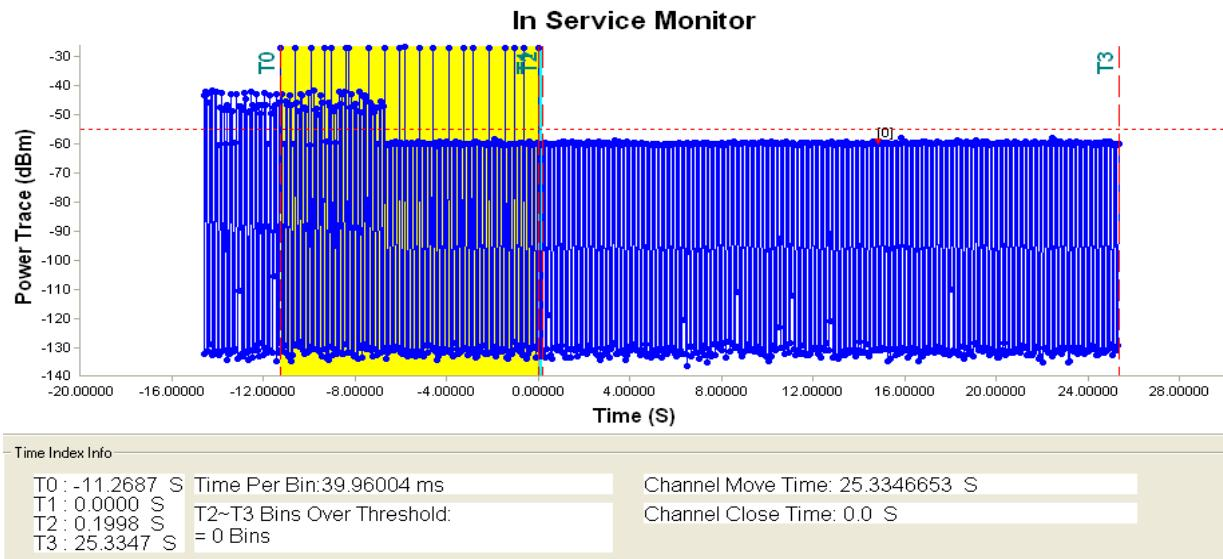
**Note:** T1 denotes the start of Channel Move Time upon the end of the last Radar burst.
