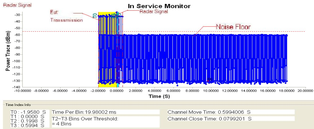
**Note:** T1 denotes the start of Channel Move Time upon the end of the last Radar burst.
