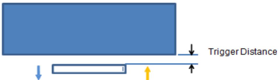
Picture: Proximity sensor triggering distances assessment (Front/Back side)
