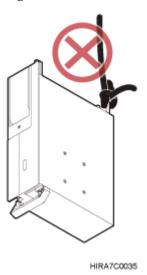
**Step 6** Hoist the RRU onto the tower, as shown in Figure 6-5. Installation engineer B pulls the lifting sling downwards, and installation engineer C pulls the traction sling outwards to protect the RRU from colliding with the tower.
