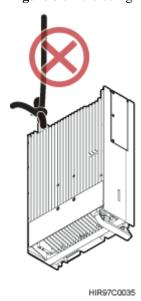
Figure 6-5 Forbidding hoisting an RRU by the traction eye only
