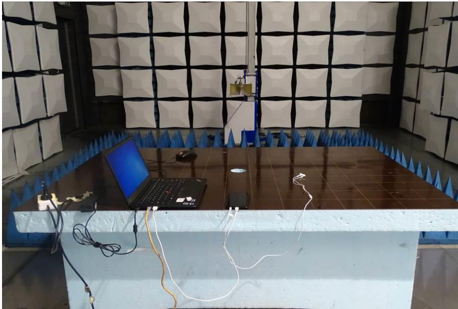
Radiated Disturbance Emissions (1GHz to18GHz)
