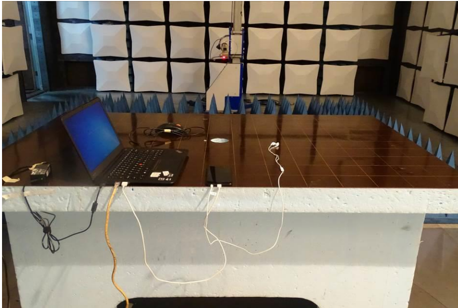
Radiated Disturbance Emissions (18GHz to 26.5GHz)
