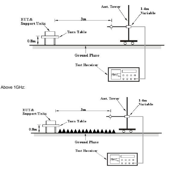
The radiated emission tests were performed at the 3 meters distance in chamber, using the setup accordance with the ANSI C63.4-2014. The specification used was the FCC Part 15.109 Class B limits.
