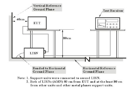
The setup of EUT is according with per ANSI C63.4-2014 measurement procedure. The specification used was with the FCC Part 15 B Class B limits.
