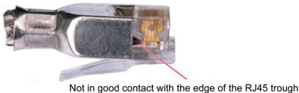
Figure 5-37 Wires not in good contact with the edge of the RJ45
