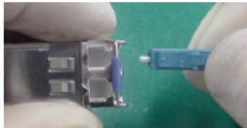
Figure 5-98 Using fibers to protect an optical module
