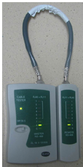
Figure 5-39 Testing the conduction and connections of wires
