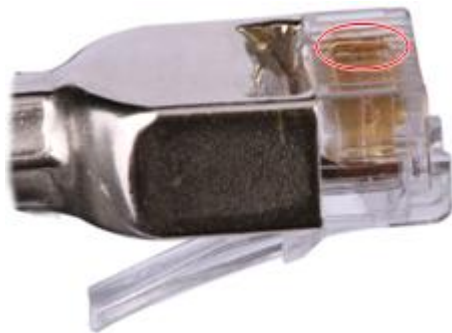
Figure 5-34 Unparallel contact strips of different heights
