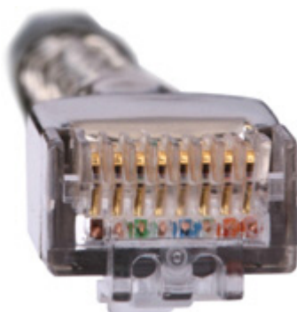
Figure 5-33 Contact strips of the same height
