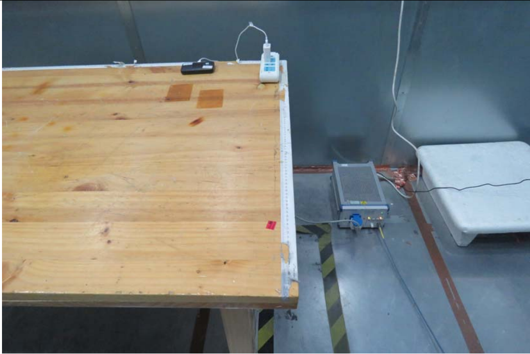
Picture 3 Conducted Emission Test Setup
