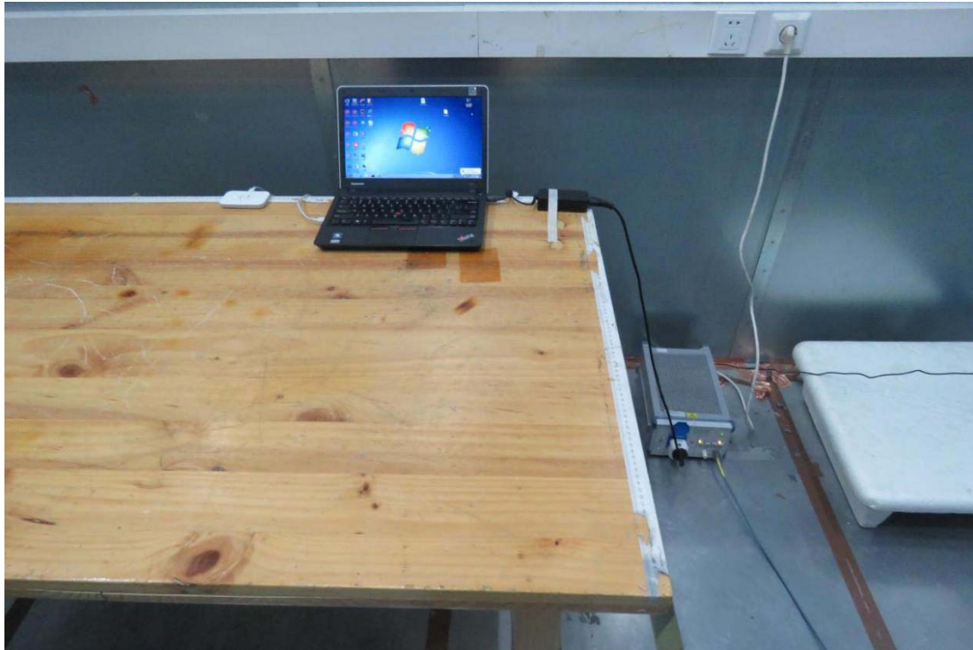
Picture 3 Conducted Emission Test Setup
