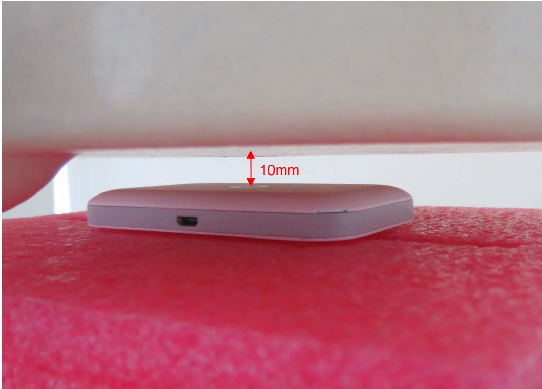
Picture 8: Back Side, the distance from EUT to the bottom of the Phantom is 10mm
