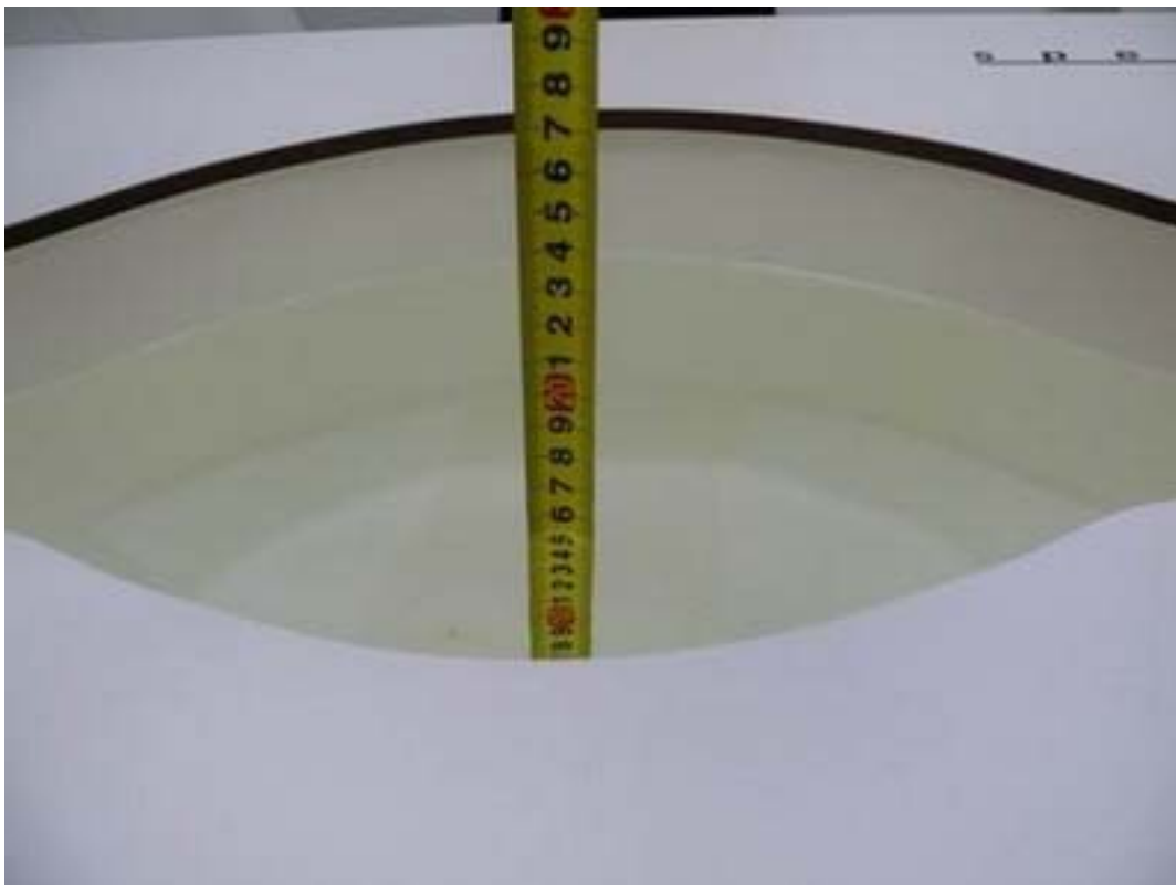
Picture 4: Liquid depth in the flat Phantom (1900 MHz, 15.2cm depth)
