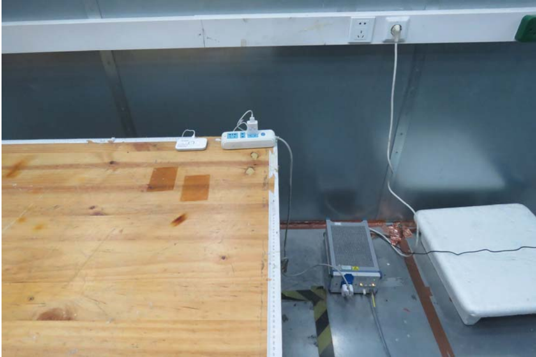
Picture 3 Conducted Emission Test Setup
