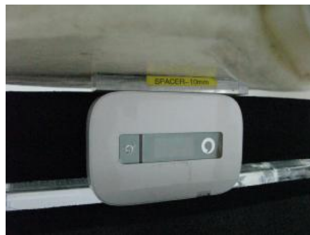
Fig.2-4 Photograph of the Hotspot status-Bottom
