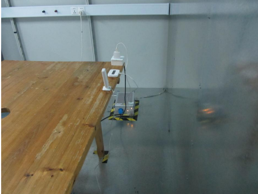
Conducted Emissions for AC Ports
