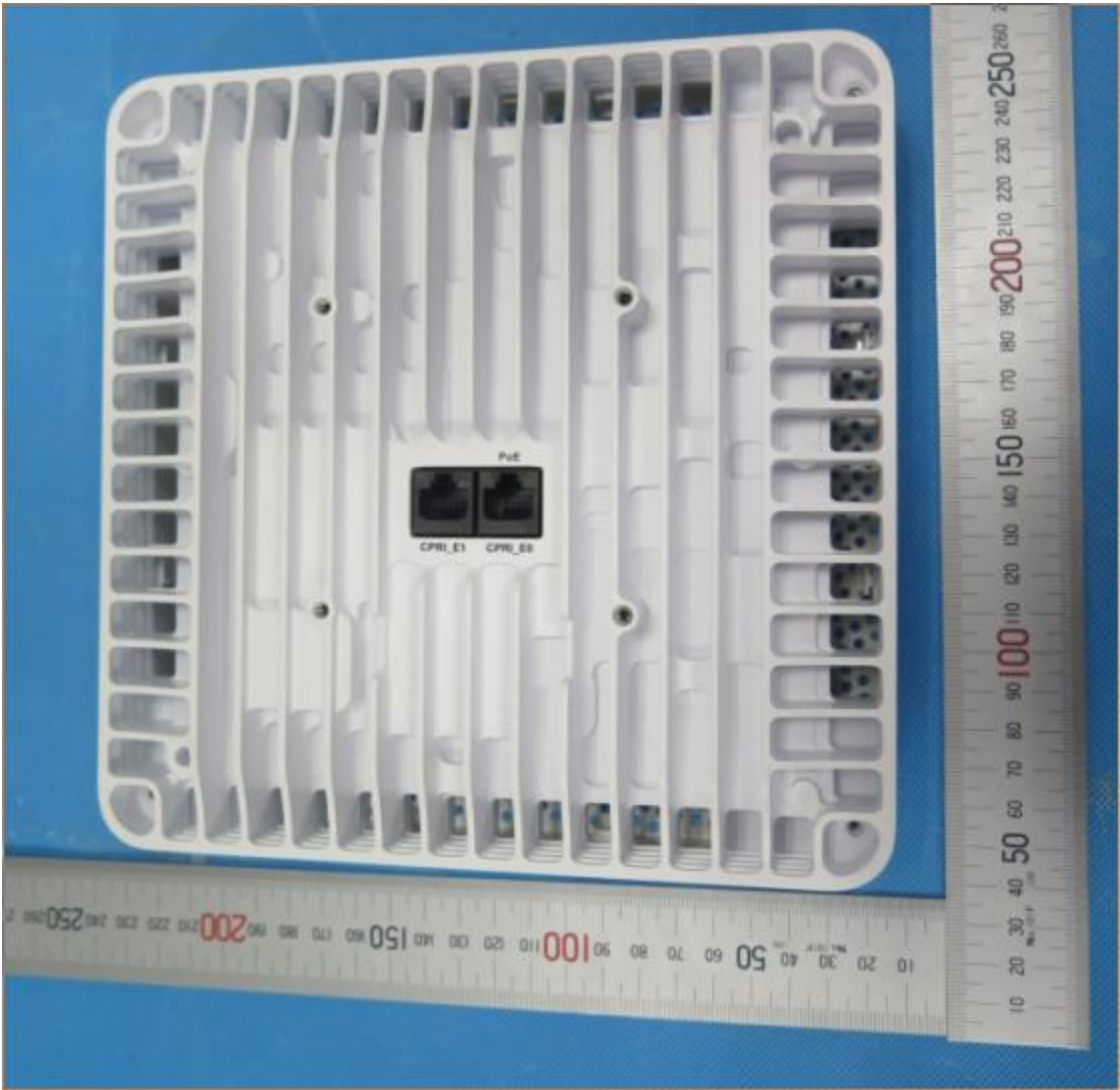
Photo-04 External -Ports
