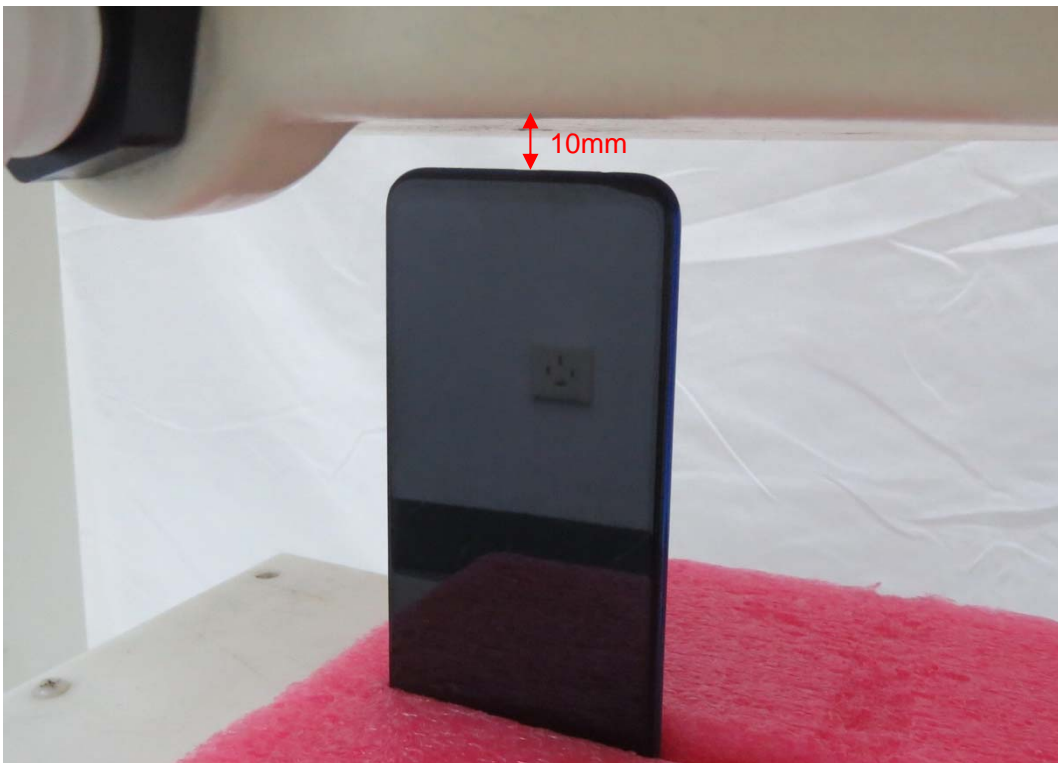
Picture 12: Bottom Edge, the distance from handset to the bottom of the Phantom is 10mm
