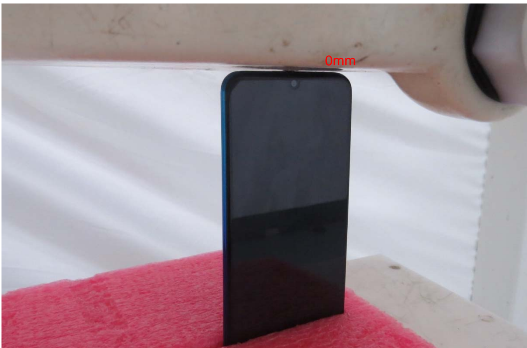
Picture 16: Top Side, the distance from handset to the bottom of the Phantom is 0mm
