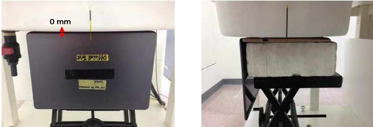
Fig.3 EUT Bottom side to flat phantom
