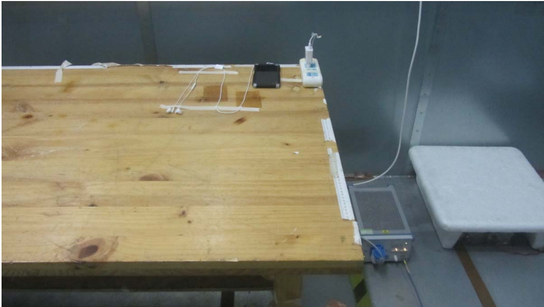
Picture 2 Conducted Emission Test Setup
