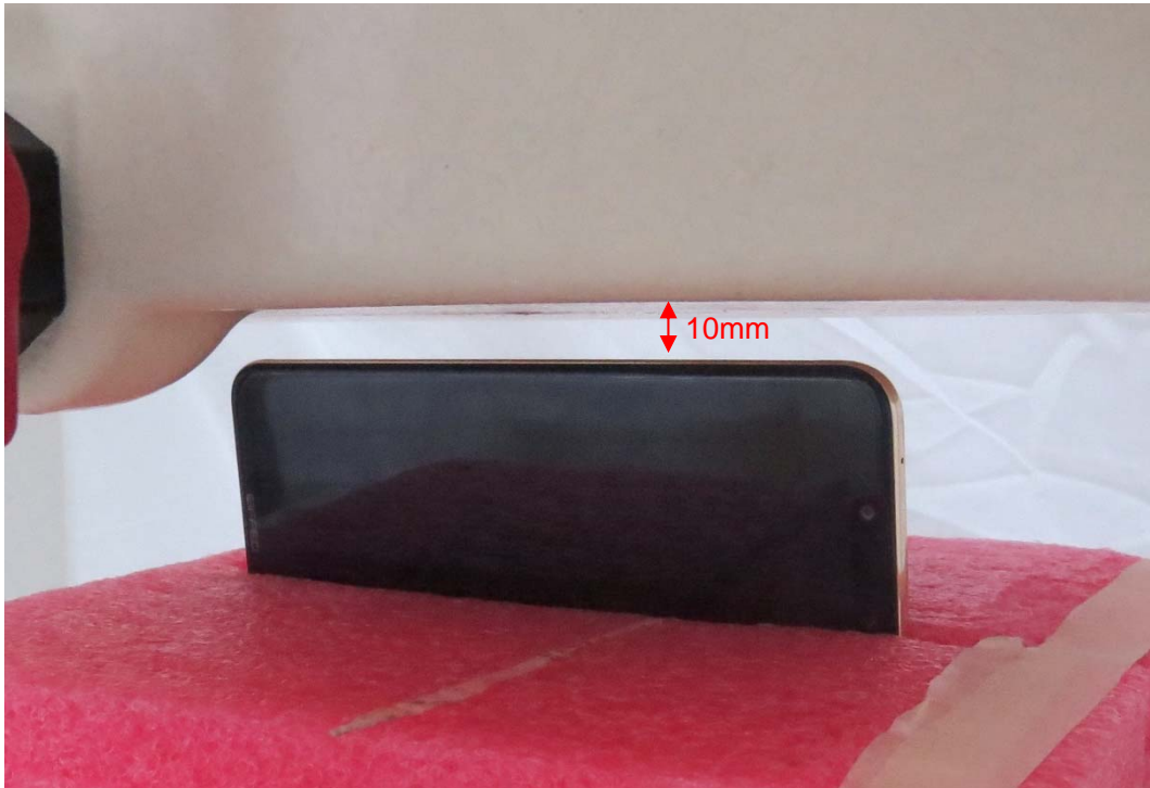
Picture 9: Left Side, the distance from handset to the bottom of the Phantom is 10mm
