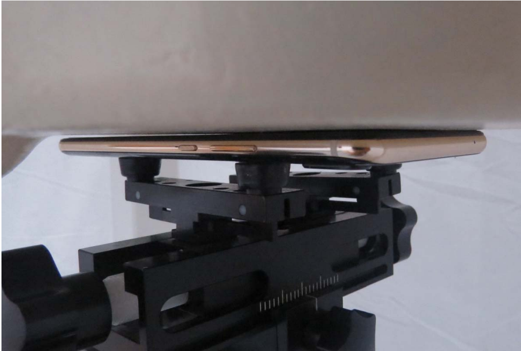
Picture 13: Back Side, the distance from handset to the bottom of the Phantom is 0mm
