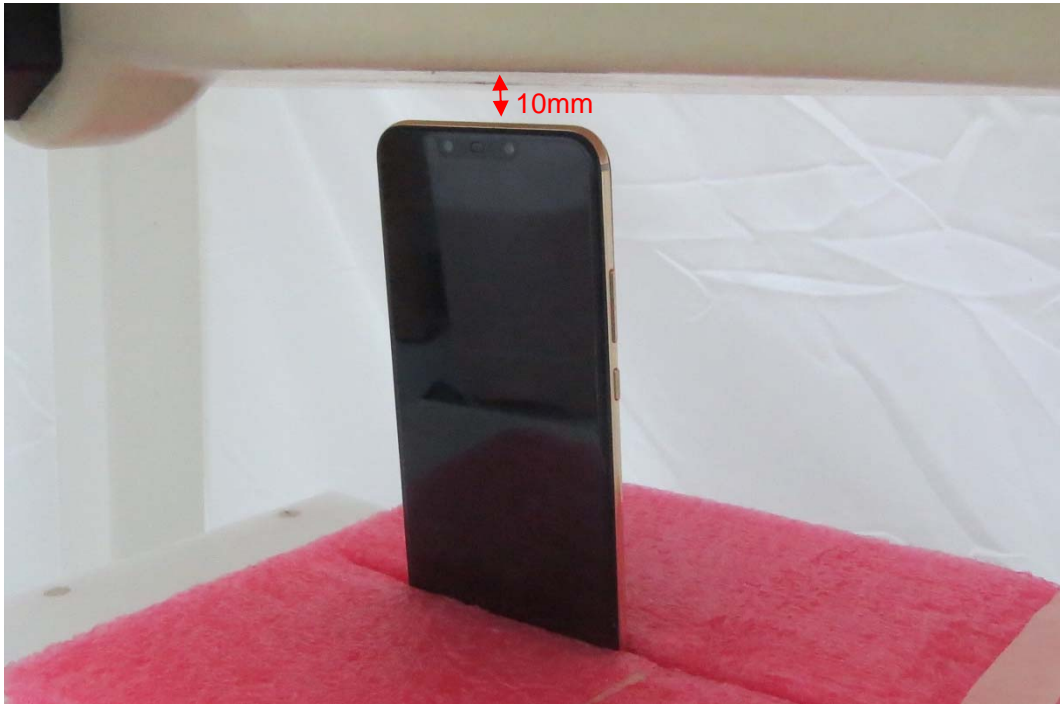
Picture 11: Top Side, the distance from handset to the bottom of the Phantom is 10mm
