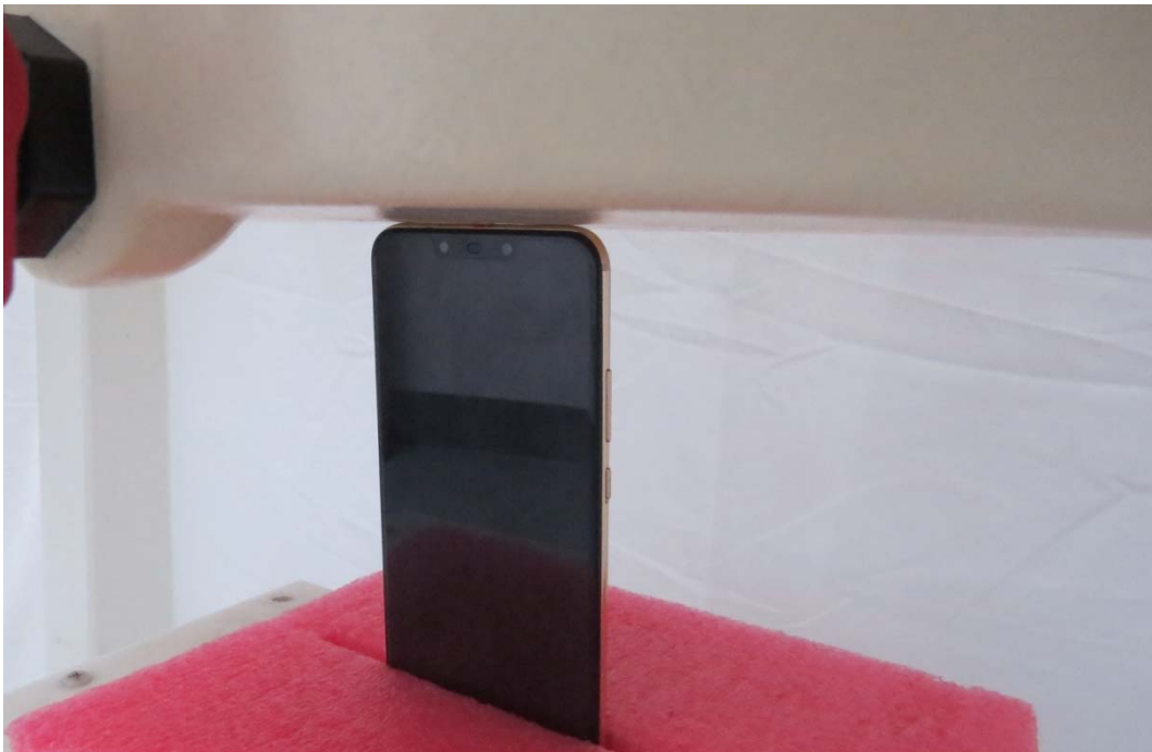
Picture 16: Top Side, the distance from handset to the bottom of the Phantom is 0mm
