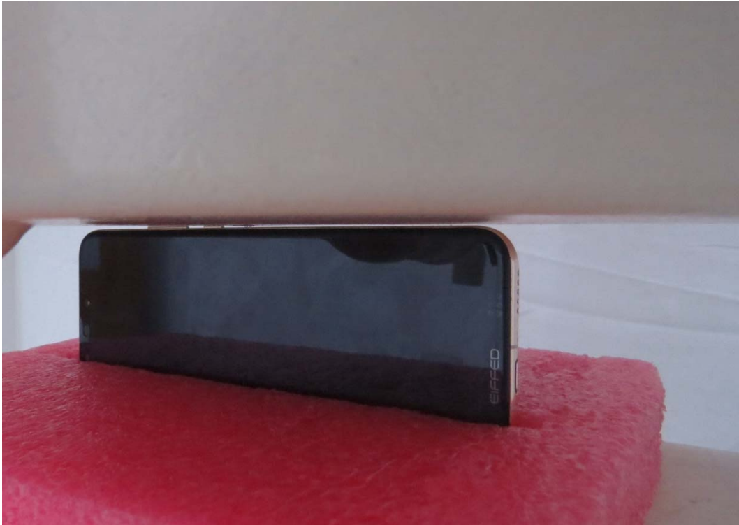
Picture 15: Right Side, the distance from handset to the bottom of the Phantom is 0mm
