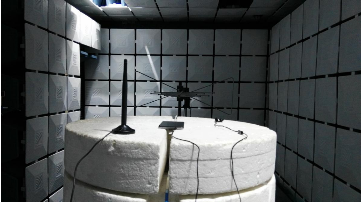
Radiated Spurious Emission (below 3GHz)
