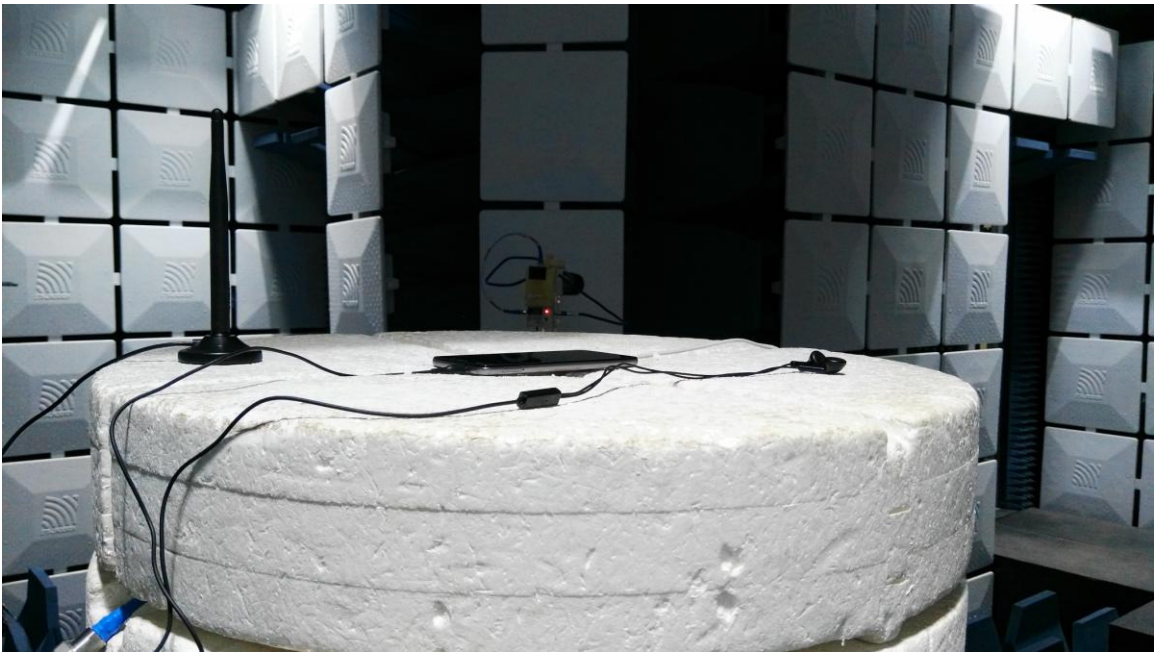
Radiated Spurious Emission (18GHz to26.5GHz)
