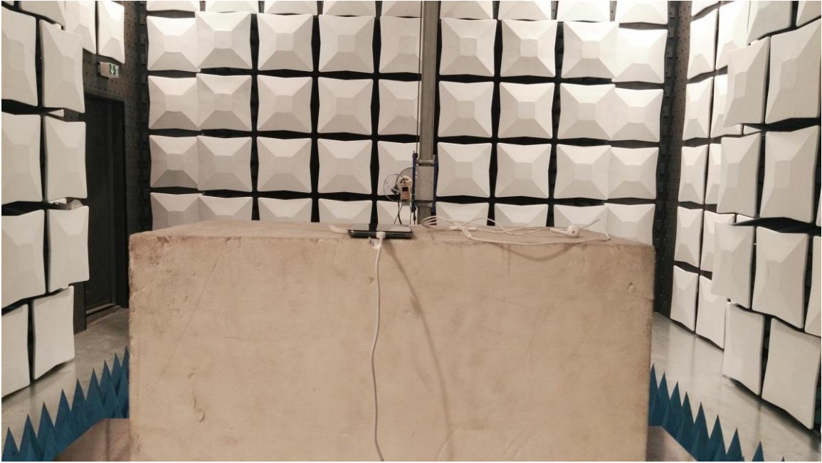
Radiated Spurious Emission (above 18GHz)
