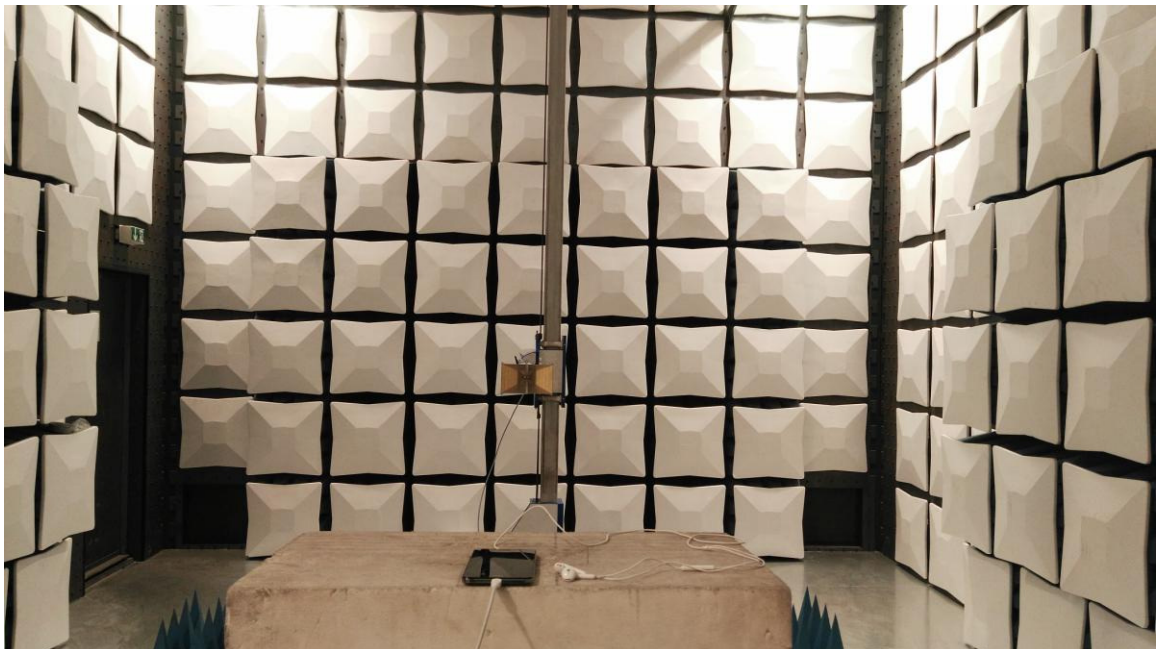
Radiated Spurious Emission (1GHz to18GHz)
