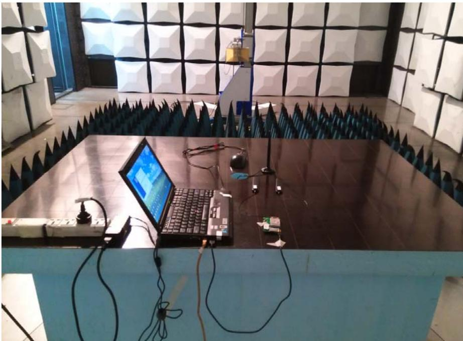
Radiated Disturbance Emissions (1GHz to18GHz)
